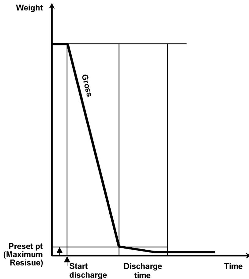
Discharge: The material is batched in discharge feed rate until the gross weight is below the maximum residue (preset point). This parameter is stored under [Preset].
