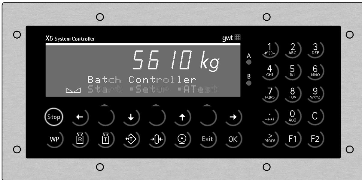
The Weight Display allows display of 7 digits for weight plus a decimal point. The weight unit can be selected as tons, kilograms, grams or lbs. The display is capable of handling two lines of alphanumeric characters in addition to the numeric output. The other symbols of the display are listed below:
