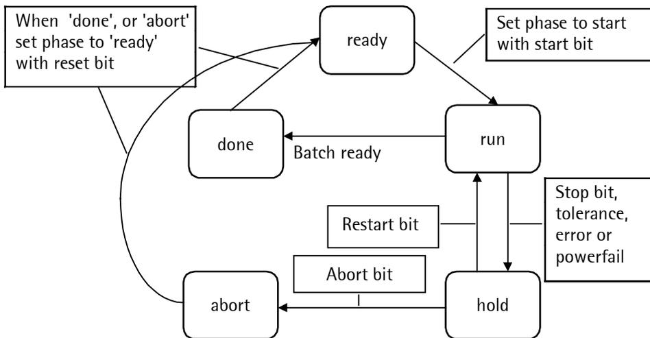
Control is via the direct control bits in byte 6. Note that the signals react only on a 0-1 transition.
