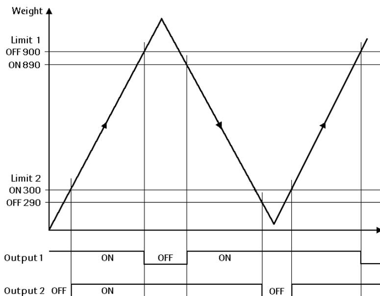
If the limit values for ON and OFF are equal the limit switch switches on, if the weight increases over the value and switches off, if the weight decreases below the value.
